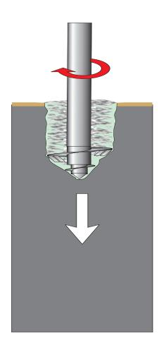
Lowering the mixing tool into the soil with 100 – 200 rpm. A substantial amount of soil gets mixed with under pressure injected suspension.
