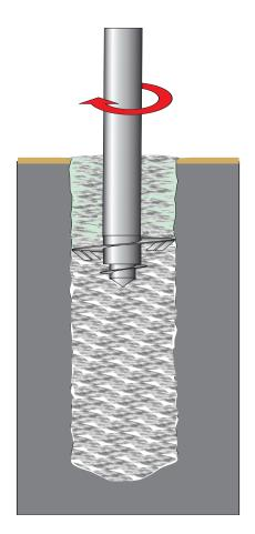
The developed mixture from soil and suspension gets mixed again during withdrawal and suspension is continuously pumped.
