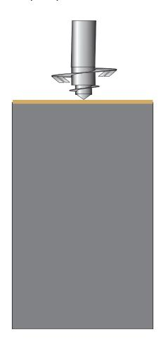
Positioning of the tooling. The mixing tool is mounted on a high revolutions ABI auger drive while the suspension supply is hooked up. (suspension= water cement mixture in various ratios)
