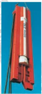
In the case of the HPH2400 and HPH6500 special off-set leg inserts can be supplied to drive larger pairs of sheet piles.
