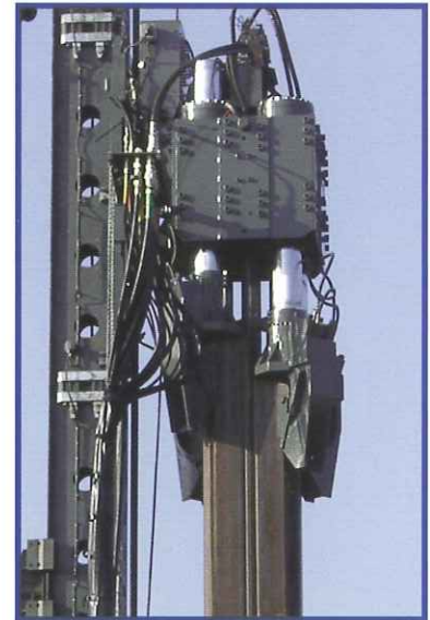
4 Cylinder Push-Pull Foundation Box Pile on Liebherr LRB255 - UK
