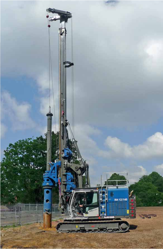
The smallest model of the DELMAG rotary drill rigs, the RH 12/140 while Kelly drilling. The machine can be transported with the rotary head and Kelly bar still attached.
