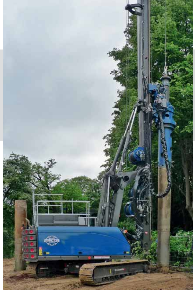
The smallest model of the DELMAG rotary drill rigs, the RH 12/140 while Kelly drilling. The machine can be transported with the rotary head and Kelly bar still attached.
