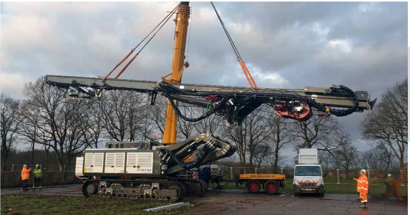
Removing the complete leader mast unit via the separable two pieces boom extension, on a drill rig RH 40. In order to reduce the transport weight of the machine, the complete leader mast unit can be removed for transport within a remarkably short space of time.
