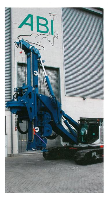
The DELMAG Kelly drill rig RH 24 in short mast version is directly derived from the recently introduced RH24 with the same performance characteristics. At maximum reach this compact unit has a working height of only 7600 mm. This allows using the rig in low head room areas like under bridges, power lines, inside buildings etc. The RH24 features a new rotary head BT 240 and offers great design details like:
