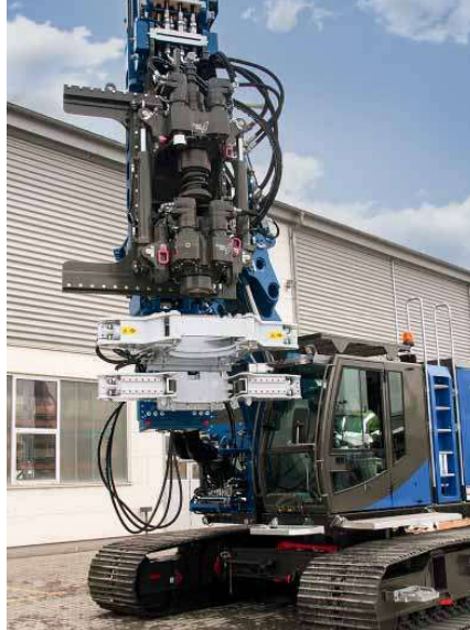
ABI MOBILRAM TM 17 with micro pile equipment, the auger drive can be moved laterally out of the drilling axis, the clamping and breaking device is used for handling the single micro pile elements.
