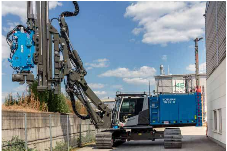
ABI MOBILRAM TM 20 LR- one machine with longer reach, primarily designed for working below or above the work platform, e. g. for pile driving elements on embankments, near roads or motorways.
