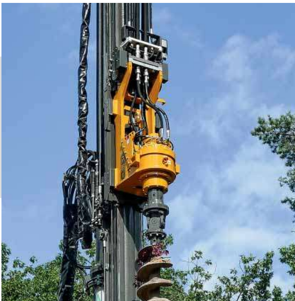
The auger drive MDBA can be used for several applications: e. g. for pre-drilling, CFA drilling as well as for soil mixing.
