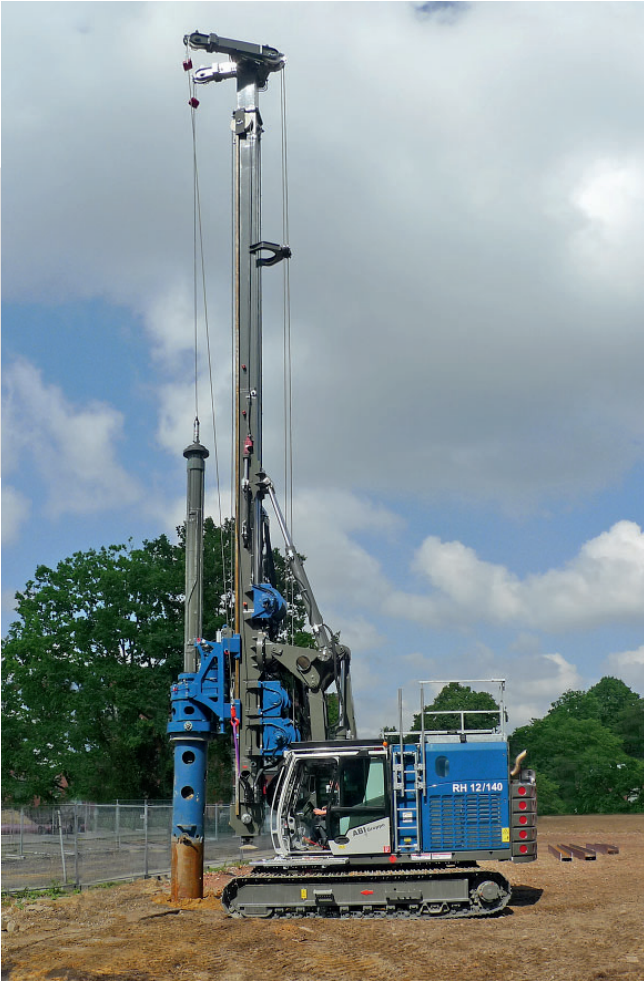
The smallest model of the DELMAG rotary drill rigs while Kelly drilling. The machine can be transported with the rotary head and Kelly bar still attached.
