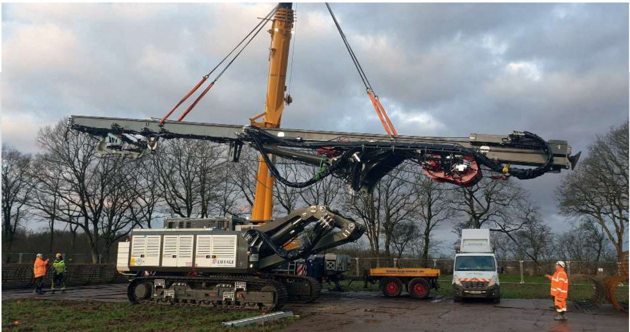
Removing the complete leader mast unit via the separable two pieces boom extension in order to reduce the transport weight of the machine, the complete leader mast unit can be removed for transport within a remarkably short space of time.
