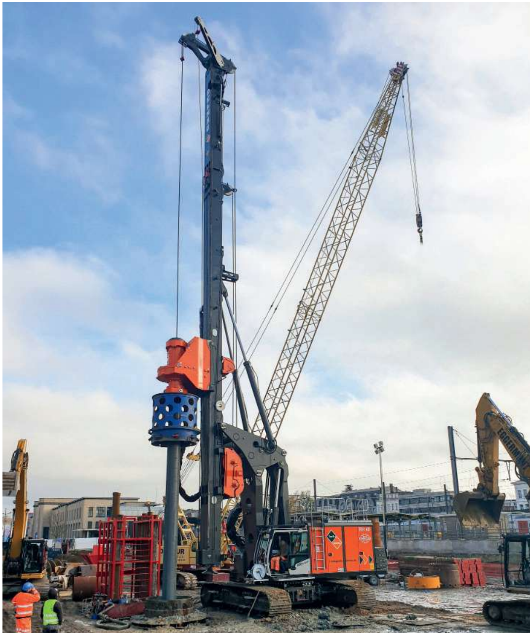
The biggest model of the DELMAG rotary drill rigs built on an ABI T110 carrier for the production of drilled piles with a diameter of 1800 mm and to a depth of 40 m using the Kelly drilling method.
